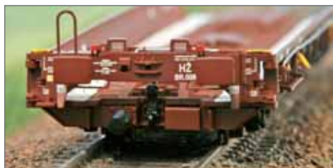
Set Rollende Landstraße HŽ composto da due carri Tipo Saadkms-z per trasporto di camion. Rollende Landstraße HŽ set composed by two Type Saadkms wagons for truck transport. Rollende Landstraße Set HŽ bestehend aus zwei Typ Saadkms-Wagen für den LKW-Transport.
