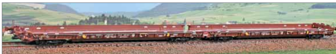
Set Rollende Landstraße HŽ composto da due carri Tipo Saadkms-z per trasporto di camion. Rollende Landstraße HŽ set composed by two Type Saadkms wagons for truck transport. Rollende Landstraße Set HŽ bestehend aus zwei Typ Saadkms-Wagen für den LKW-Transport.
